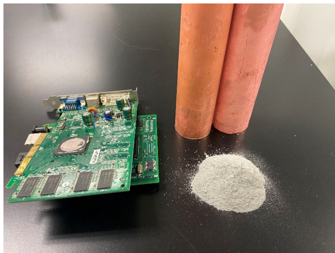
Figure 1: Copper and tin oxide (powder) recovered from PCBAs
